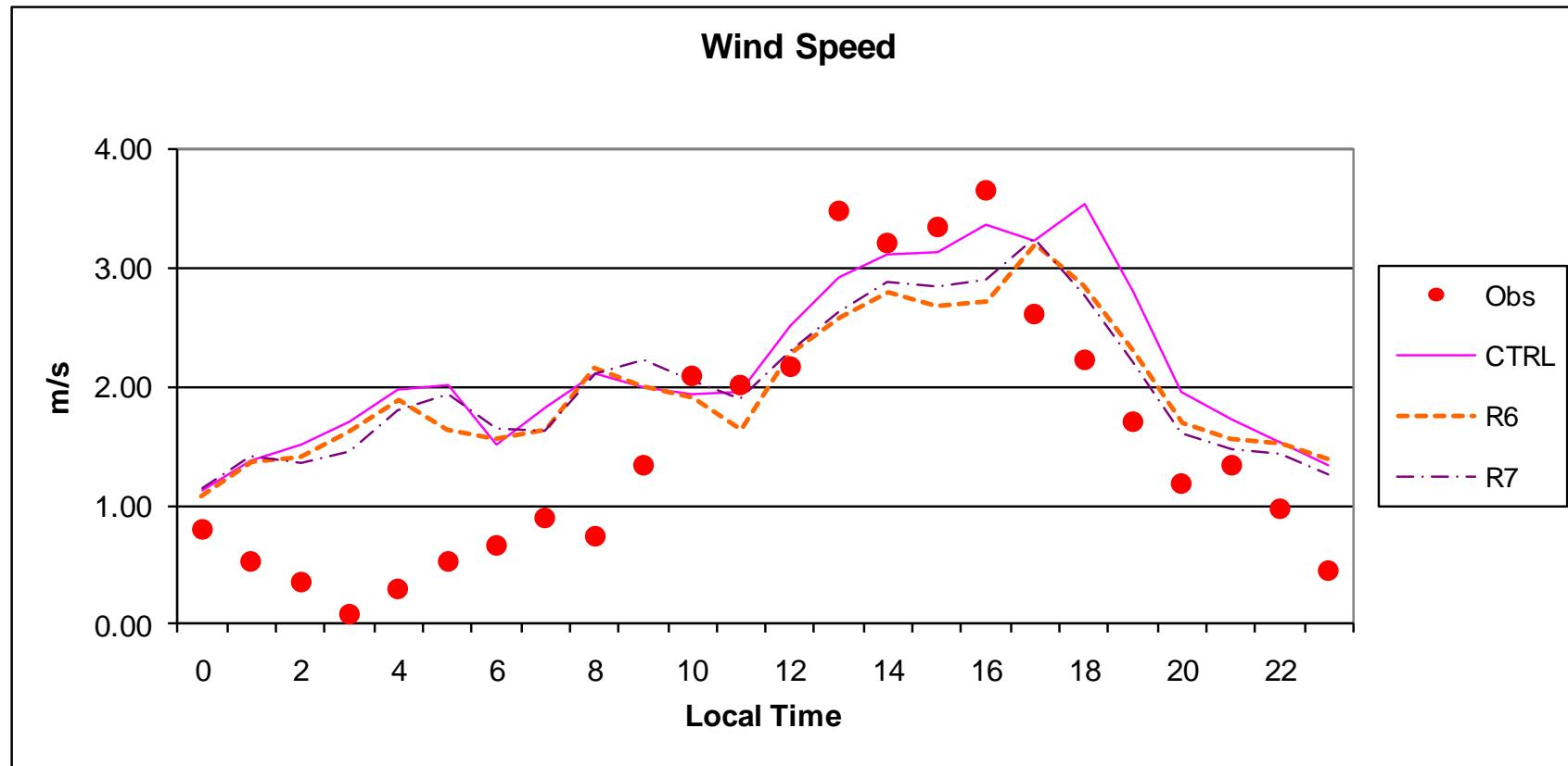
**R6:** Suburban,  $z_0 \text{ urb} = 1.5 \text{ m}$ ,  $z_0 \text{ suburb} = 0.7 \text{ m}$ ,  $z_0 w = 0.1 \text{ cm}$
